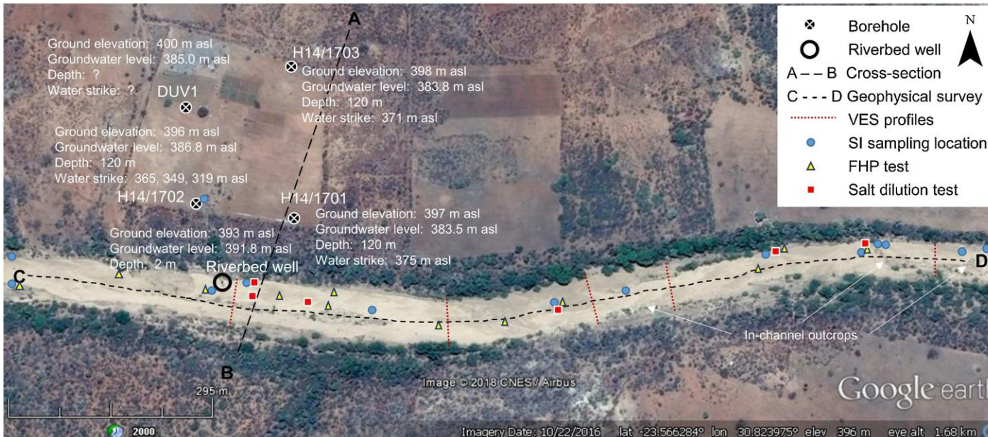
Plan of the Molototsi sand river site showing borehole information, testing and sampling locations (SI = stable isotope, FHP = falling head permeameter) and the geophysical survey lines (VES = vertical electrical sounding) along the Molototsi sand river (Walker et al. 2018)
